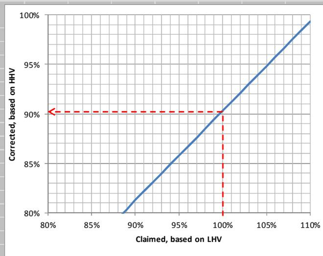
Line shows example with 100% claimed efficiency based on fuel LHV equating to 90.3% efficiency based on fuel HHV.
